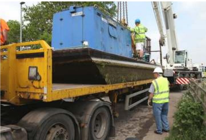
The Mudlark is 35’ long, 8’ wide, 7’ 3” high and weighs in at 15 tonnes
