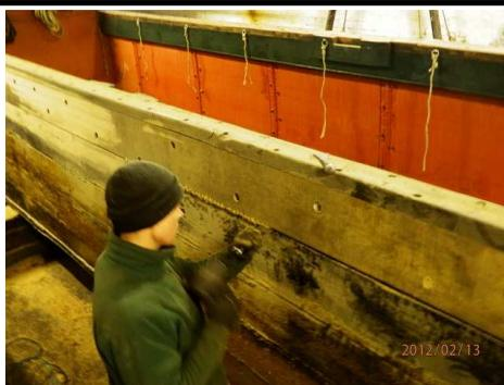
*Caulking seams of the new side plank*
