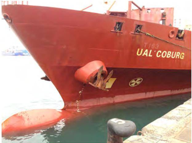
At slow speed, the bulbous bow is a hindrance. Maersk are removing bulbs from ten of its ships and the
