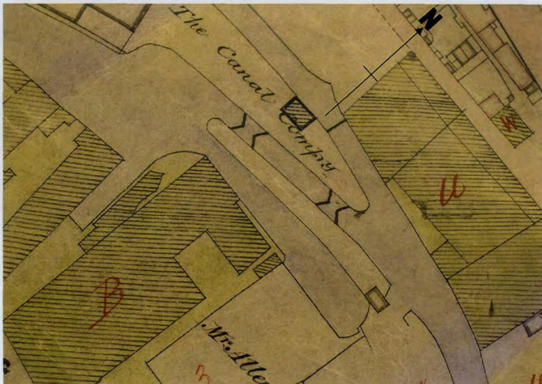
Map of 1858 showing double-gated junction lock with the River Salwarpe alongside the original Droitwich Basin. From survey of 1854 by Webb & Buck. © Worcester Record Office BA 1840
