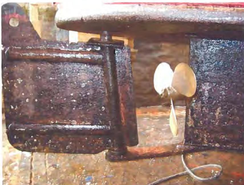
Figure 4.3 Narrow boat with propeller and rudder configuration
