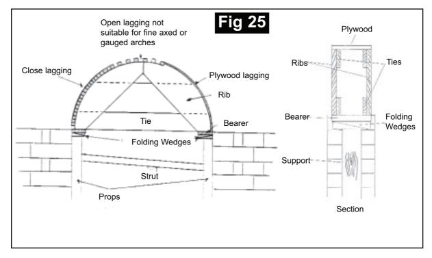
RIBS are the semi - circular members which are used to make the shape of the arch.
