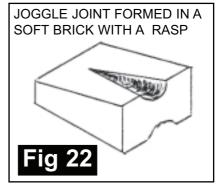
**JOGGLE JOINTS** : in a few cases when cutting arches, after the voussoirs have been cut to shape, a deep groove is cut into all the
