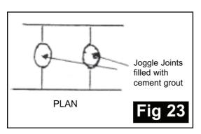
bricks on both sides of the bed joint, fig 22, if they are soft bricks then you can use a coarse half round file. If you are using hard bricks then a comb hammer can be used. When all the voussoirs have been laid in the arch the joggle joint can be filled with a strong (1:1) cement /sand mix, fig 23.
