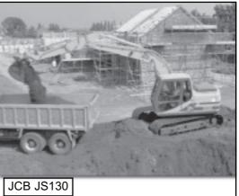
Truck positioned as close to machine centre line, with work angle kept as small as possible be kept to 15<sup>o</sup> either side of the centre of the machine or about equal to under carriage width. Trucks should be positioned as close as possible to the machine centre line. This avoids excessive time slewing to load behind you.
