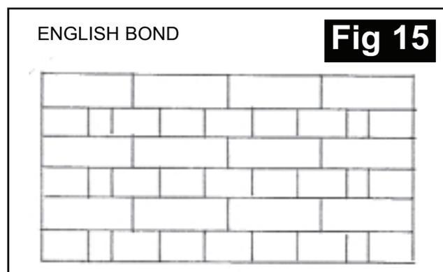
quarter bat can be placed at the quoin but only in the stretcher course. This is a very strong bond, with no straight joints appearing in any part of the wall. The face of the wall being monotonous to look at, it is used in walls where strength is preferable to appearance and always used in conjunction with engineering bricks, *fig 15*.
