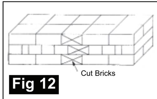
6. If the wall is such a length that a cut must be introduced, the cut must be placed in the middle of the wall this is known as broken bond, see *fig 12*.
