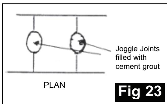
bricks on both sides of the bed joint, *fig 22*, if they are soft bricks then you can use a coarse half round file. If you are using hard bricks then a comb hammer can be used. When all the voussoirs have been laid in the arch the joggle joint can be filled with a strong ( 1:1 ) cement /sand mix, *fig 23*.
