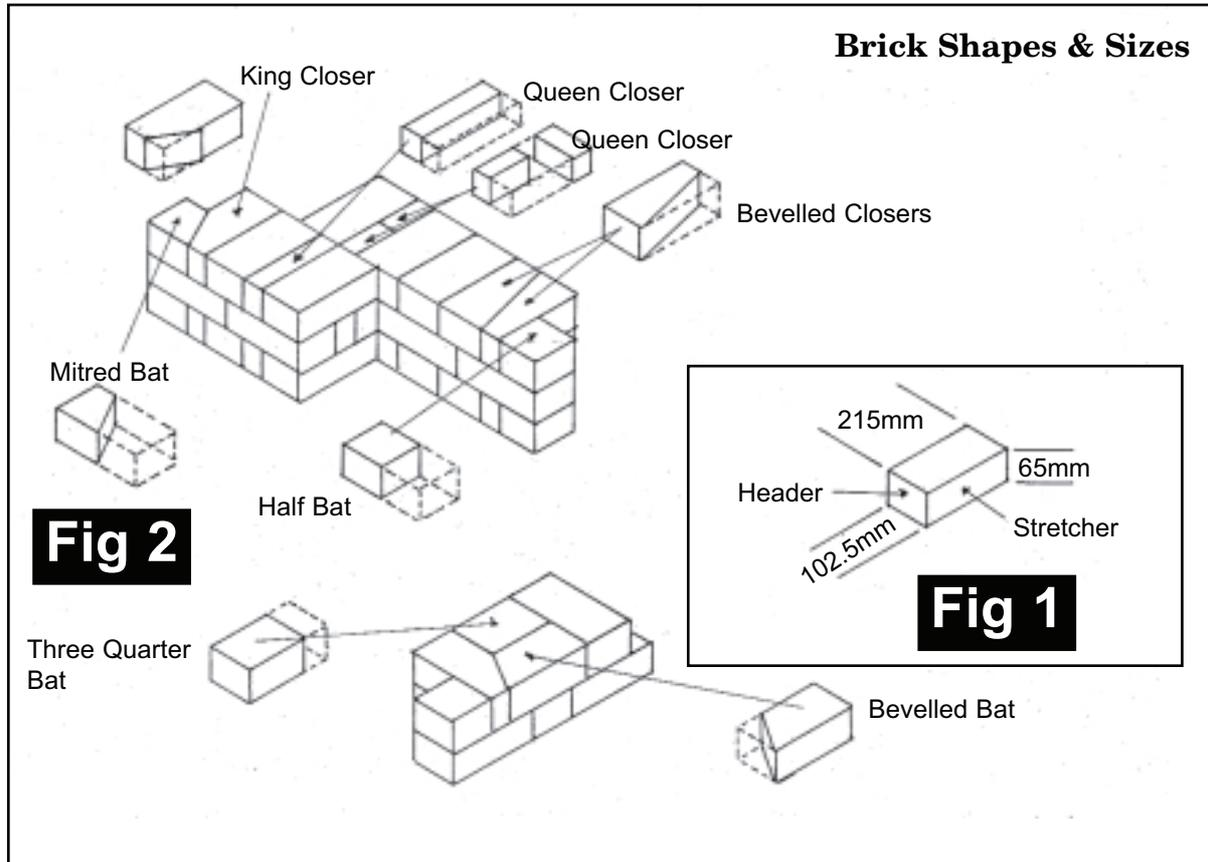
A three-quarter bat which has a minimum size of 150mm long by 100mm wide
