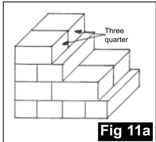
4. When using new bricks on an existing wall there is no way you will keep up with the existing bond, because all you will end up with is wide perp joints or several cuts in the wall which look very unsightly. The ideal way is to ignore what is below and start afresh, except where you are joining onto an existing wall, i.e. maintain the individual courses of headers and stretchers.
